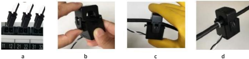
Figure 2-13 5A/2mA, 100A/40mA, 200A/40mA or 400A/40mA SCCT Installation
